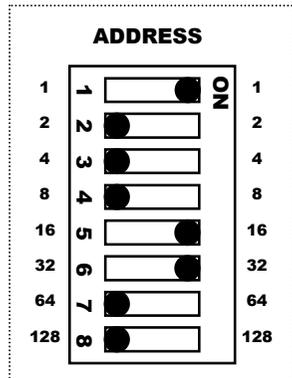
Set the address by adding up the numbers on the left or right side. For example to set address 24, set switch 4 and 5 to the 'ON' position. Switch 4 gives you 8 and setting switch 5 adds 16 which gives the address 24. In the example to the left, the address is set to 49 (1 + 16 + 32).
