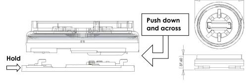
To release, push Release Tool into holes in rim of sounder unit and slide the product in the reverse direction.
