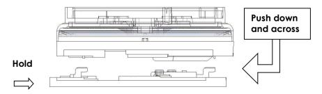
To release, push Release Tool into holes in rim of sounder unit and slide the product in the reverse direction.
