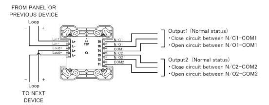
Relay Module contains two isolated sets of Form-C contacts, which operate as a DPDT switch. The module allows the control panel to switch these contacts on command. No supervision is provided for the relay contacts.
