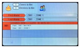
The LCD gives all the alarm information, such as the time & date of the alarm, the address, the device type, the device label, and the zone it is allocated to.
