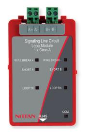
The plug-in NMP-SLC module provides power for and handles communications to the analogue addressable devices. The SLC continuously monitors the analogue values of all devices and displays this value, in the Panel Real Time menu, to assist with potential fault finding.
