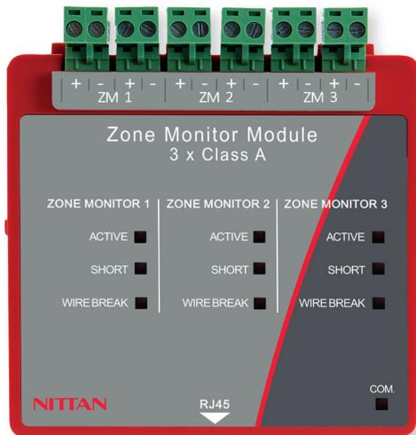
The NMP-ZMA is a three zone monitor module that is designed to be DIN mounted inside of an Evolution UL control panel. It's powered and interfaced to the Evolution UL NMP via a RJ45 connection.
