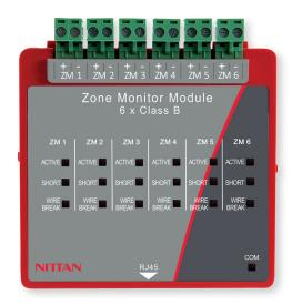
The NMP-ZMB is a six zone monitor module that is designed to be DIN mounted inside of an Evolution UL control panel. It's powered and interfaced to the Evolution UL NMP via a RJ45 connection.
