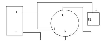
UB-4 / STB-4SE Bases RIL must be 6v, 2mA max
