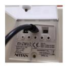
The mini USB style connector can be plugged into the front of the installed module.
