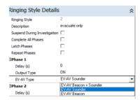
Any EV-AV2 type devices included within the group operation will follow the setting for the ringing style. Note it will not alter the operation of other types of sounder device driven by the same ringing style they will follow the evacuation or alert operation set. If Beacon only is selected, then other types will not respond. The ringing style can then be used in the cause and effects line as required.
