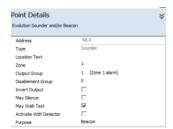
Note: - if the May Silence check box is left ticked for any sounder within a group for this purpose then a design error message will be given and an upload will be blocked.
